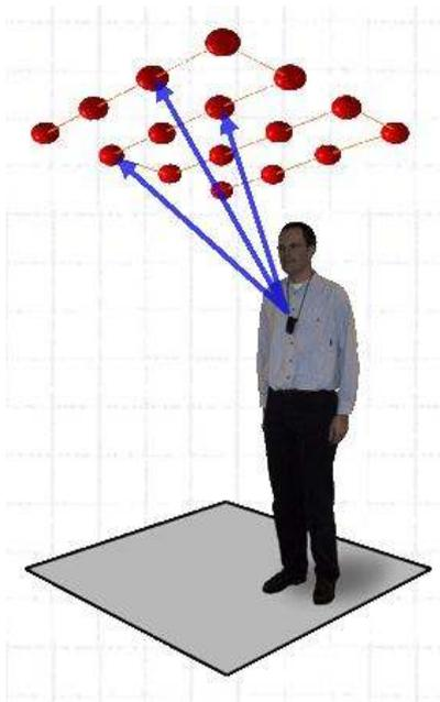
Figure 3: How triangulation works with Active Bat [11]
