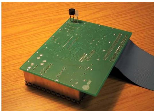
Figure 4: Receiver used to detect ultrasonic signals.
