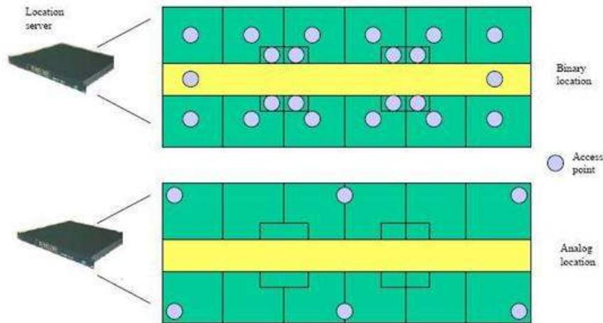
Figure 8: The two types of AP arrangement [11]
