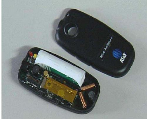
Figure 5: AT&T developed Active Bat sensor
