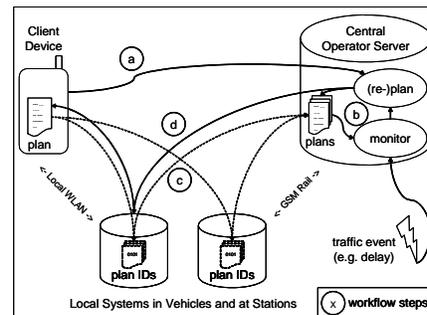
Figure 3: Proposed system architecture for operator-driven replanning
